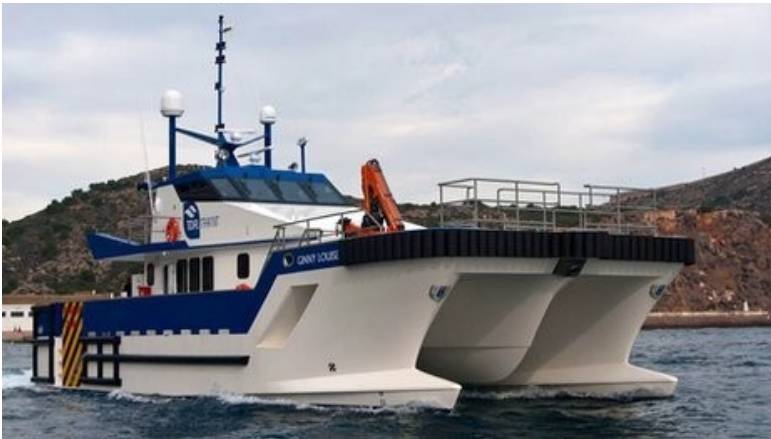
The Ginny Louise can achieve 27 knots and is equipped with a moon pool for camera surveys
