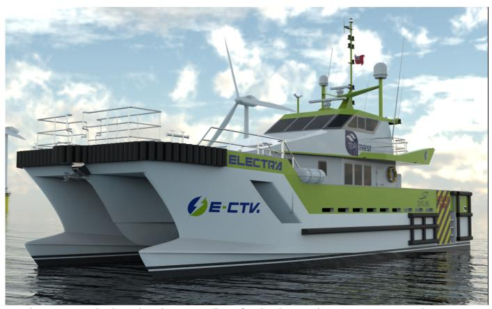
Over the next 15 months, the UK-based company will retrofit a diesel-powered Mercurio 20-metre vessel, *Ginny Louise*, with over 2 MWh of battery capacity, electric motors, and propulsion pods.
